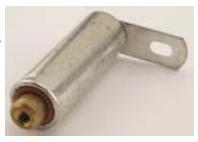
A simpler way of checking if it's a bad condenser is to remove the distributor cap, body and rotor. Make sure the points are closed. Turn the ignition switch on and place the high tension wire (from centre of coil) about one-half inch from any convenient ground on the engine. Push points open with a screwdriver then close. The spark should jump the gap with a sharp crack and a straight line. The spark should have a blue tinge.
