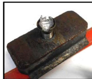
Drilled-out screw reinserted in field coil pole shoe
