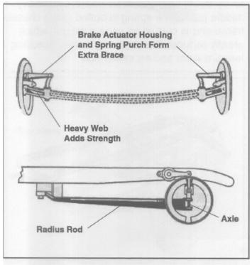
radius ball is used to secure the end of the radius rods to the bottom of the bell housing. This forms a rigid construction for the front axle, eliminating any twist action at the front axle.
