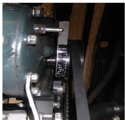
Shows the Nu Rex timing guide plus the harmonic balancer pulley ex Murray Horne which was another item that resulted in a transformation of the motor.
