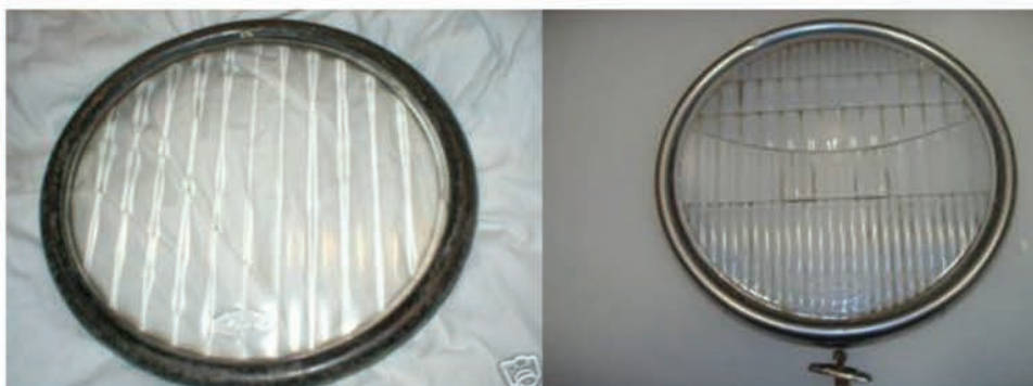
Comparison of Model A Headlight Lenses 1928 Lens (left) has vertical "flutes" - 1929-1931 Lens has different design Both have the Ford Script in an oval at the bottom of the lens
