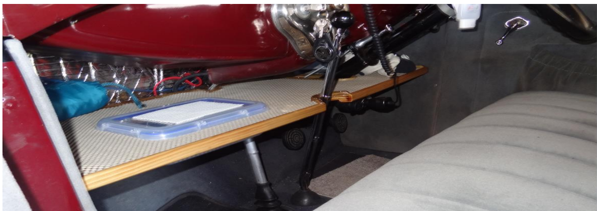
The shelf in place showing the indent for the gear stick gear stick and container for those small items.
