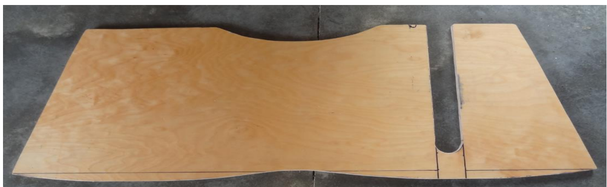
The cut-out shelf showing the slot for the steering column.
