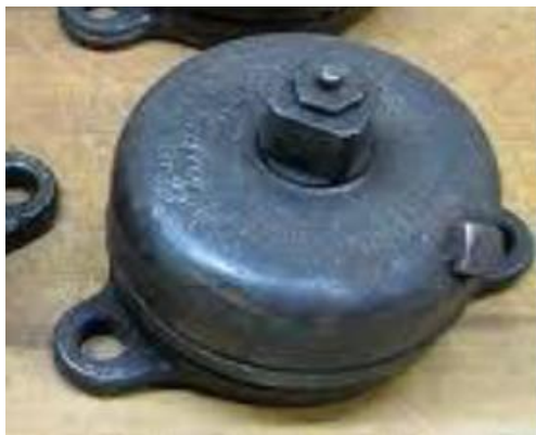
Shock absorber all put back together and ready for painting and installation.
