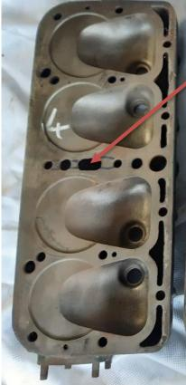
During October 1929 the centre oval opening to the water jacket was added for better cooling. Heads 4, 5 and 6 like this are all marked with W1. The one on the left is cracked through the three holes in the centre.
