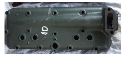
Heads 9, 10 and 11 have the diamond mark. This mark is found on castings made in the Ford factory for spare parts and industrial engines for some years after Model A production ceased. Legend has it that these are stronger parts, but according to <u>www.fordgarage.com</u> (well worth a visit) the only advantage is that they were built to the latest design at the time and are just that bit younger.
