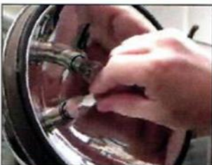
2. Push in slightly and rotate clockwise ("tighten") until the LED locks into position.
