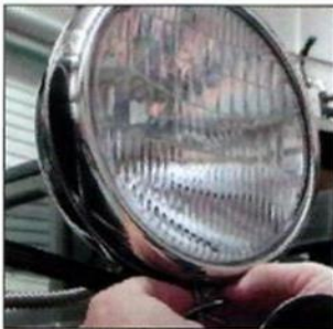
1. Push the spring-loaded headlight lens keeper back and down, releasing the lens and retaining ring
