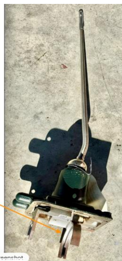
Enlarged fork/ fingers for the second gear synchronizer
