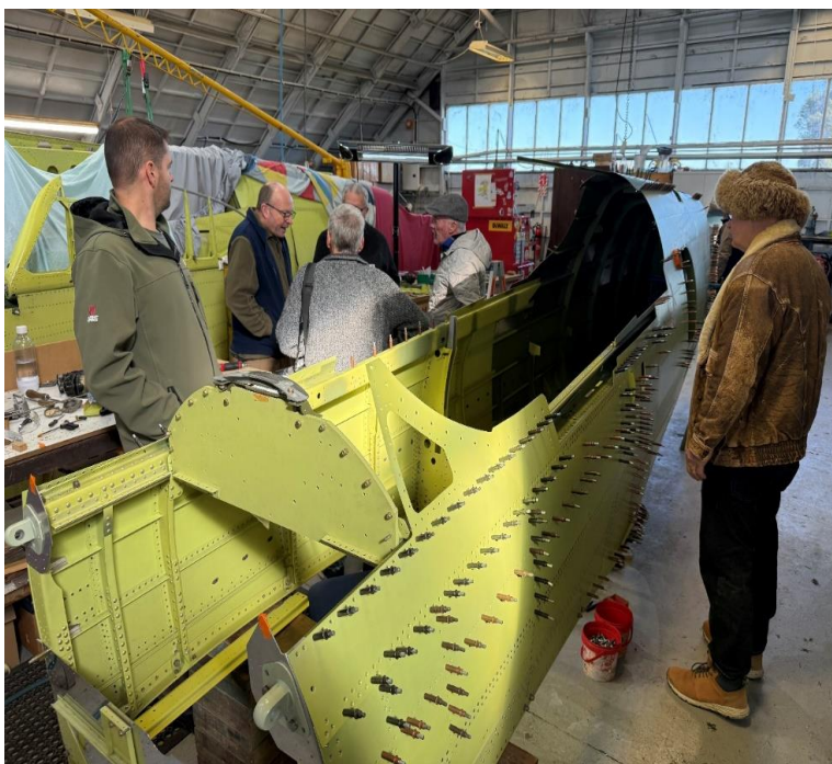
Cockpit area of P40 under construction. The big Allison engine will be at the front of this fuselage.
