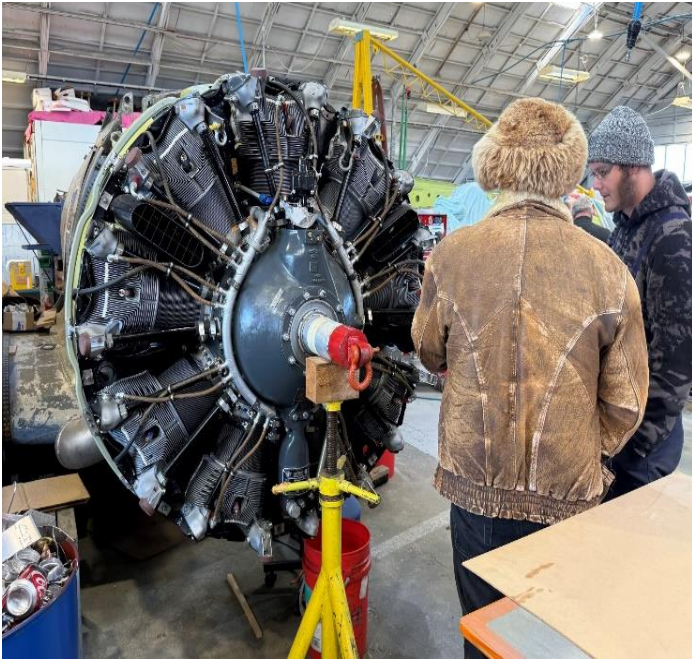
Wright Cyclone radial engine for Doubtless Dive Bomber
