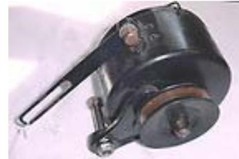
An ohmmeter can be used to check the generator field windings. The 5 brush powerhouse should read about 3 ohms, the 3 brush powerhouse about 2 ohms and the Autolite style about 1 to 1 ½ ohms. I like to test field coils by using a 6-amp battery charger with an amp meter. A 5 brush powerhouse should show about 2 amps draw across the field windings when 6 volts is applied, the
