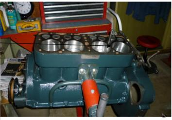
The area between #3 and #4 cylinder is a common place for a blown head gasket.
