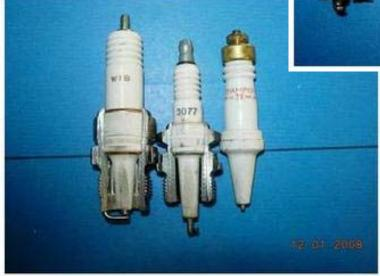
The picture to the left shows a comparison of the W18, and the Original 3X with the 3077/TT11. As can be seen, the porcelain cone is significantly longer than the W18 which means it is a hot-hot plug which may be used for an oil burner or a rich runner. If you have a bad running car, the first thing to check is what plugs you have AND does it run a little rich (probably not very good mileage either). Try the W18's.
